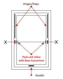
**Bow-Constrictor** must be fitted centrally at the points X-X to achieve the best seal
